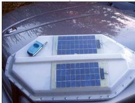
The OCS is truly an install-it-and-forget-it device. The internal battery with solar charging allows years of service-free performance.
